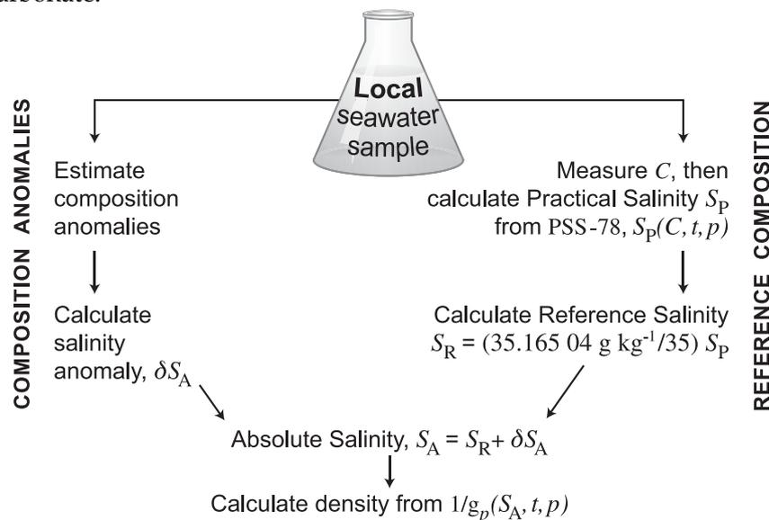
**Figure 1.** A sketch indicating how thermodynamic quantities such as density are calculated as functions of Absolute Salinity. Absolute Salinity is found by adding an estimate of the Absolute Salinity Anomaly  $\delta S_A$  to the Reference Salinity.
