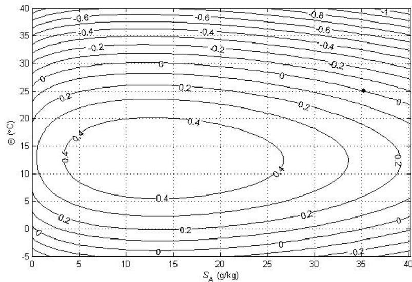
**Figure A.16.1.** Contours (in °C) of a variable which illustrates the non-conservative production of entropy  $\eta$  in the ocean.
