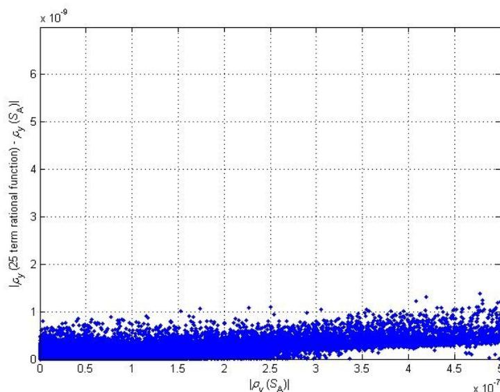
**Figure A.30.1.** The northward density gradient at constant pressure (the horizontal axis) for data in the world ocean atlas of Gouretski and Koltermann (2004) for  $p > 1000$  dbar . The vertical axis is the magnitude of the difference between evaluating the density gradient using the 25-term expression Eqn. (A.30.1) instead of using the full TEOS-10 expression, using Absolute Salinity  $S_A$  as the salinity argument in both cases.
