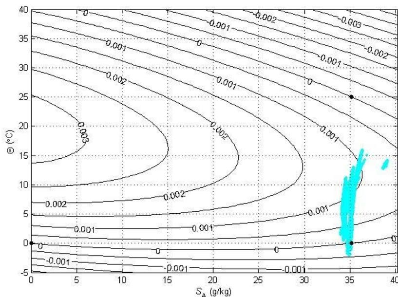
**Figure A.18.1.** Contours (in  $^\circ\text{C}$ ) of a variable that is used to illustrate the non-conservative production of Conservative Temperature  $\Theta$  at  $p = 600$  dbar. The cloud of points show where most of the oceanic data reside at  $p = 600$  dbar. The three points that are forced to be zero are shown with black dots.
