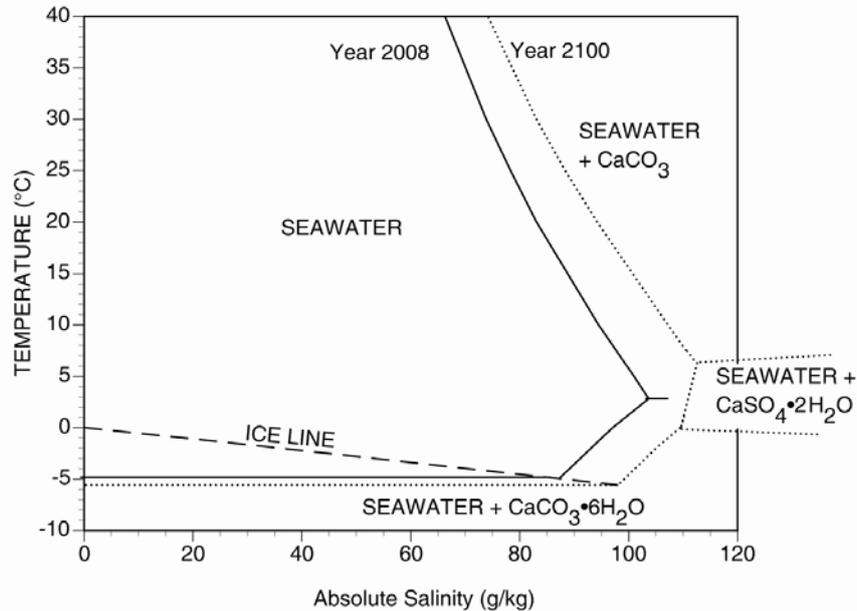
**Figure 3.** The boundaries of validity of the Millero *et al.* (2008a) composition at  $p = 0$  in Year 2008 (solid lines) and potentially in Year 2100 (dashed lines). At high salinity, calcium carbonate saturates first and comes out of solution; thereafter the Reference Composition of Standard Seawater of Millero *et al.* (2008a) does not apply.
