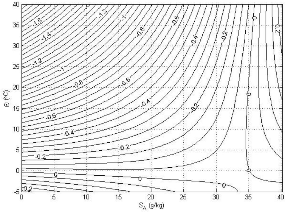
**Figure A.17.1.** Contours (in  $^{\circ}\text{C}$ ) of the difference between potential temperature and Conservative Temperature  $\theta - \Theta$ . This plot illustrates the non-conservative production of potential temperature  $\theta$  in the ocean.
